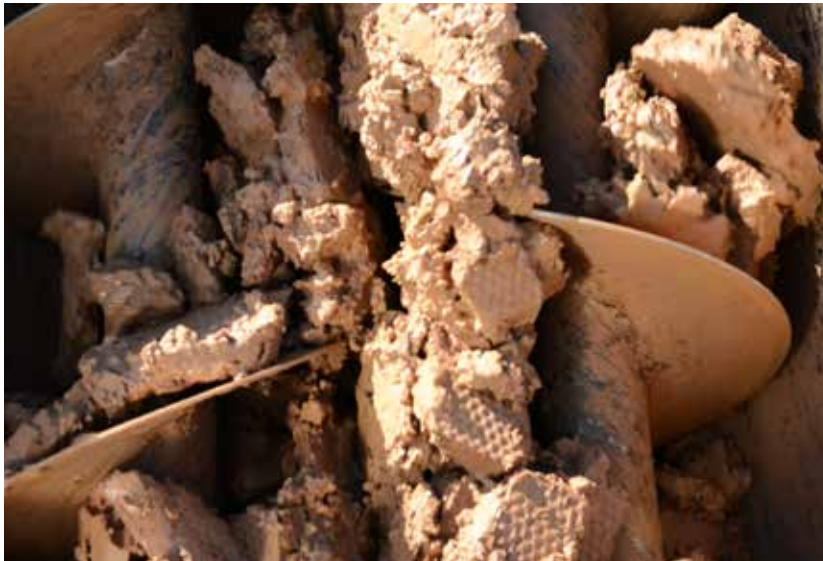
The screw conveyor below the filter press to extract the dry mud
